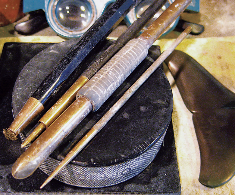
HANDSTONING: Brass pencils work well to manually apply the “telltale.” WORKBENCH: The sticks start large at the back and gradually work their way down to different bowls. Fine and super fine grits have their own bowl to avoid grit transfer.
