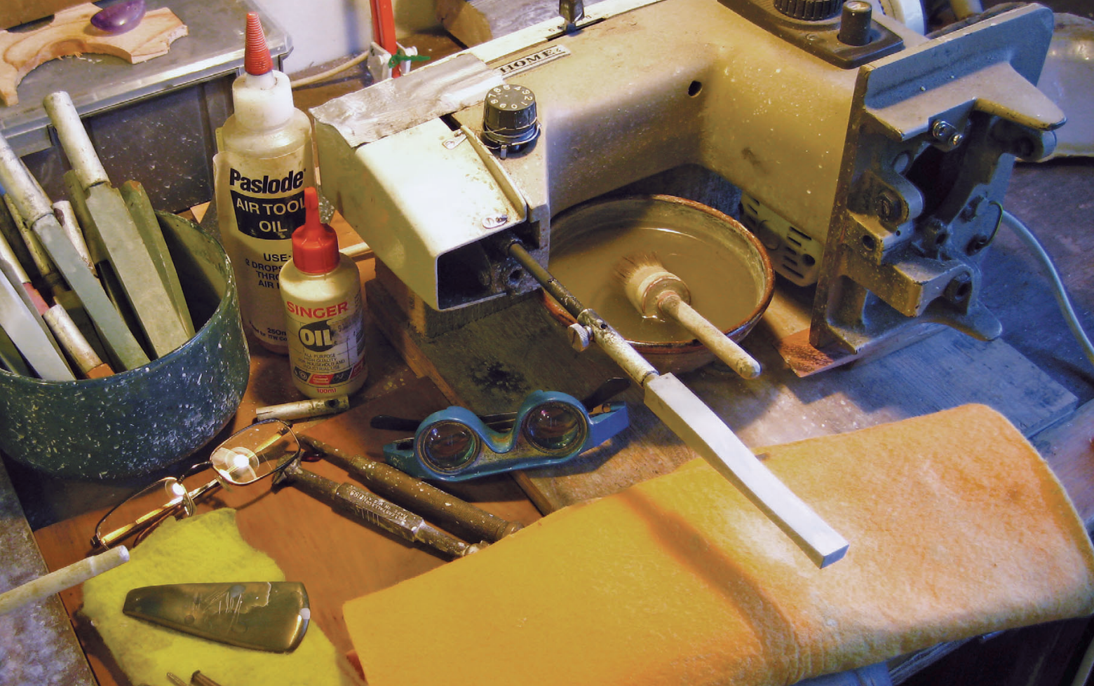
CHOPFILE: It is simple to change the sticks. Abrasive sticks can be rotated in their aluminum holders to give more profiles. The limited use of water means only sponges are needed. Oil is a regular necessity. Note the sewing machine, on its side, retooled as a chopfiller.
