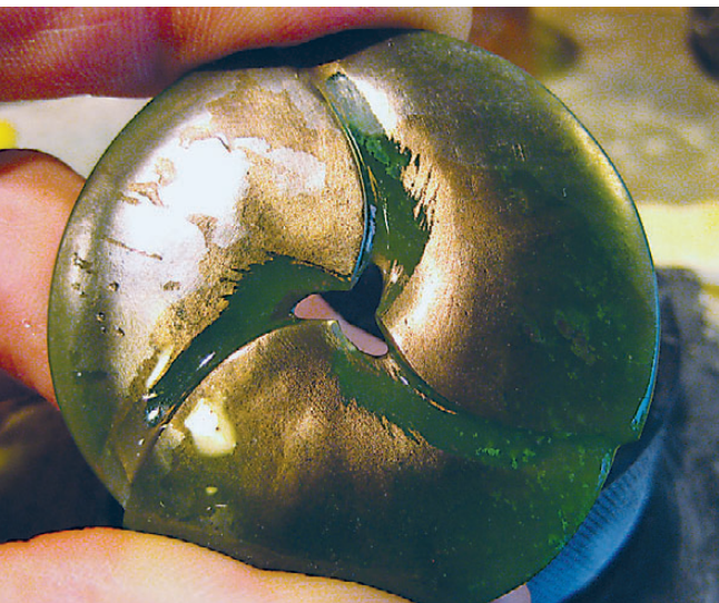
HANDSTONING: Washed down, the "telltale" clearly shows where you have been and where to cut next.
