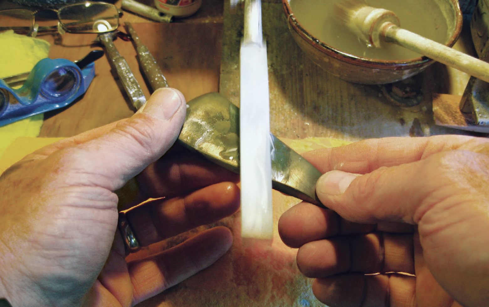
CHOPFILING: Hold the piece up gently with a little water and work up a cutting slurry. Note the brass "telltale" on the celt pendant being worked and that the workpiece is held below the abrasive stick.
