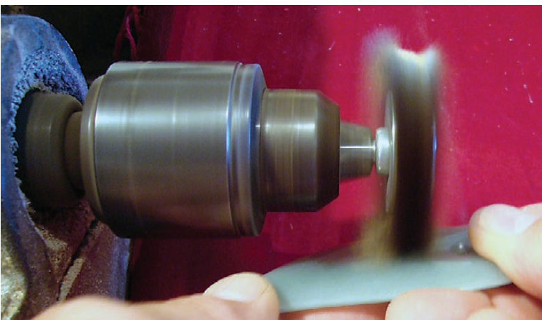
APPLYING TELLTALE: The brass brush coats the stone with the "telltale." The point carver is a basic shaft with a Jacobs chuck on the end, a versatile bit of gear I use to drive many cutting, sanding and polishing points. TELLTALE CUT OF CHOPFILE: After one direction, turn through ninety degrees to cut off the tops of the first cut with the second. Adze blade pendant ( Hei Toki ) of New Zealand nephrite, Pounamu in Maori, of blue gray ( Inanga ).
