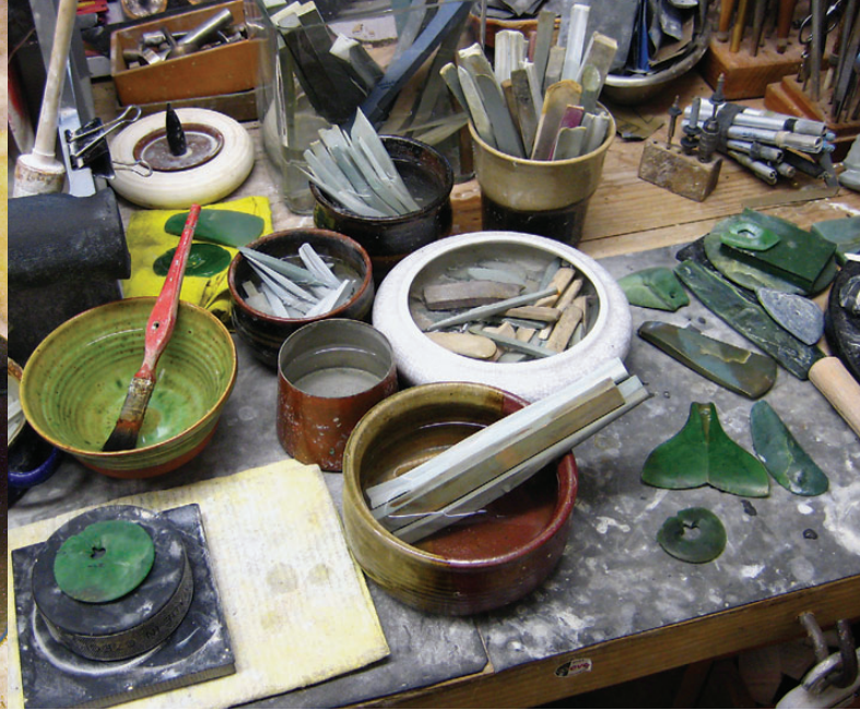
HANDSTONING: Brass pencils work well to manually apply the “telltale.” WORKBENCH: The sticks start large at the back and gradually work their way down to different bowls. Fine and super fine grits have their own bowl to avoid grit transfer.
