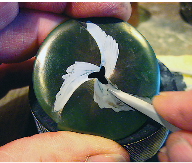
HANDSTONING: The abrasive stick quickly works its way into the groove. The cutting slurry can be easily seen here, which is why I say you have to get used to working blind.
