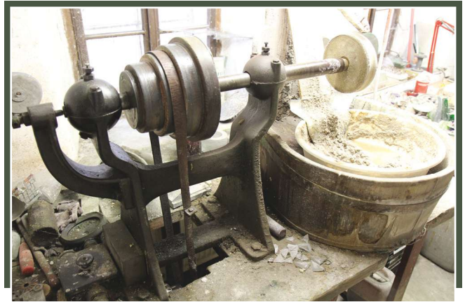
GRIND WHEELS OF VARIOUS GRITS AND SIZES. GLASS CUTTERS LATHE found in Kasalý's workshop. Note the water spout above the cutting wheel to carry away ground glass particles. Below: KASALY IN A SEPARATE WORKSHOP where he and Eva Kasalá make mosaic glass. Here he is holding two designs of glass murals. KASALY'S STUDIO. Photographs by Patrick R. Benesh-Liu.
